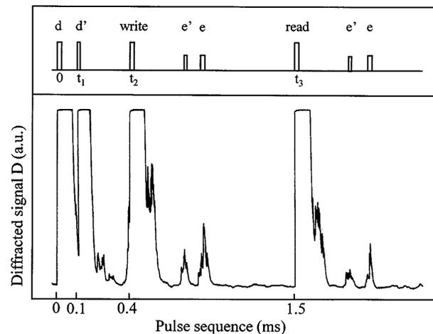
Fig. 3. Two-bit optical data storage by frequency-selective time-domain stimulated spin echo based on EIT at 6 K: d, d', data; e, e', echoes.
