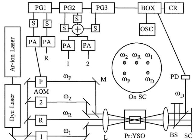
Fig. 2. Schematic of the experimental setup for frequency-selective time-domain stimulated spin echo by EIT: AOM, acousto-optic modulator; BOX, boxcar averager; BS, beam splitter; CR, chart recorder; L, lens; M, mirror; OSC, oscilloscope; PA's, rf power amplifiers; PD, photodiode; PG's, pulse generators; S's, rf switches; SC, screen.
