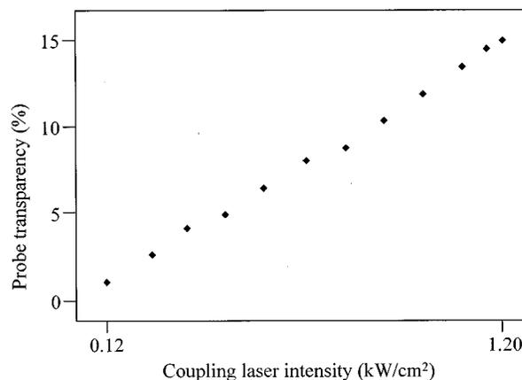
Fig. 5. Probe transparency versus coupling laser intensity.
