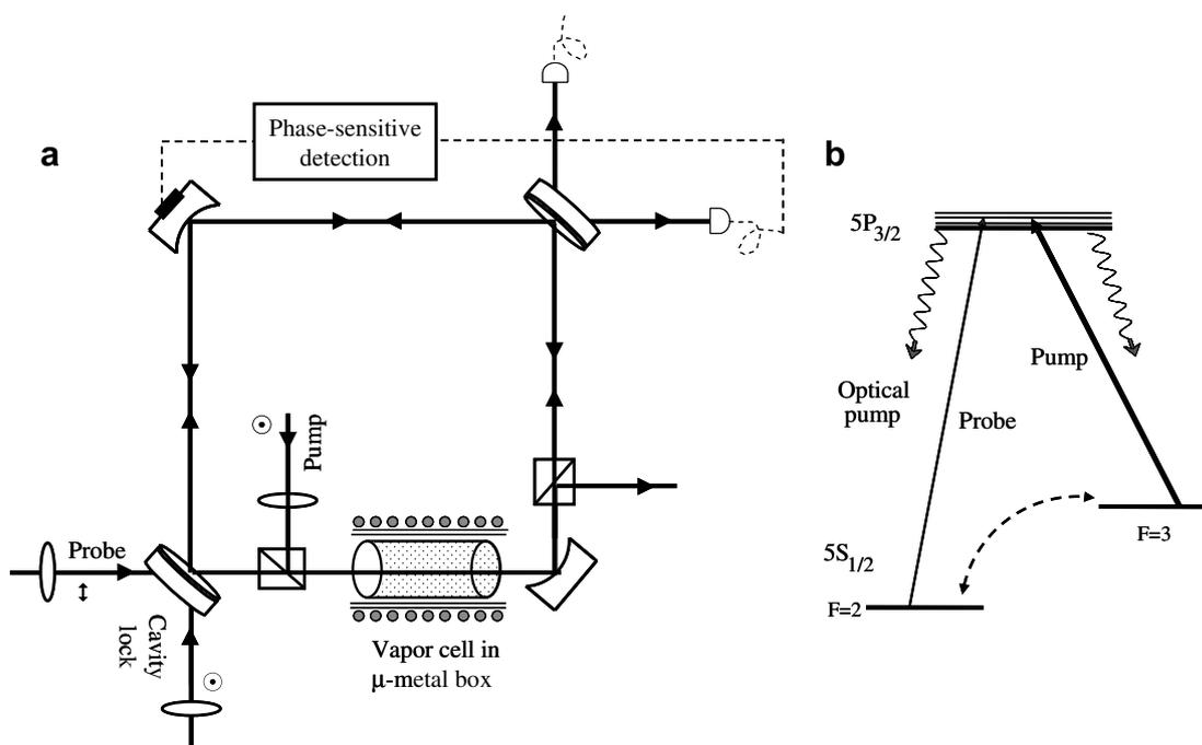
Fig. 1. (a) Schematic of experimental set-up, (b) two-photon transitions used in  $^{85}\text{Rb}$   $D_2$  line for EIT.
