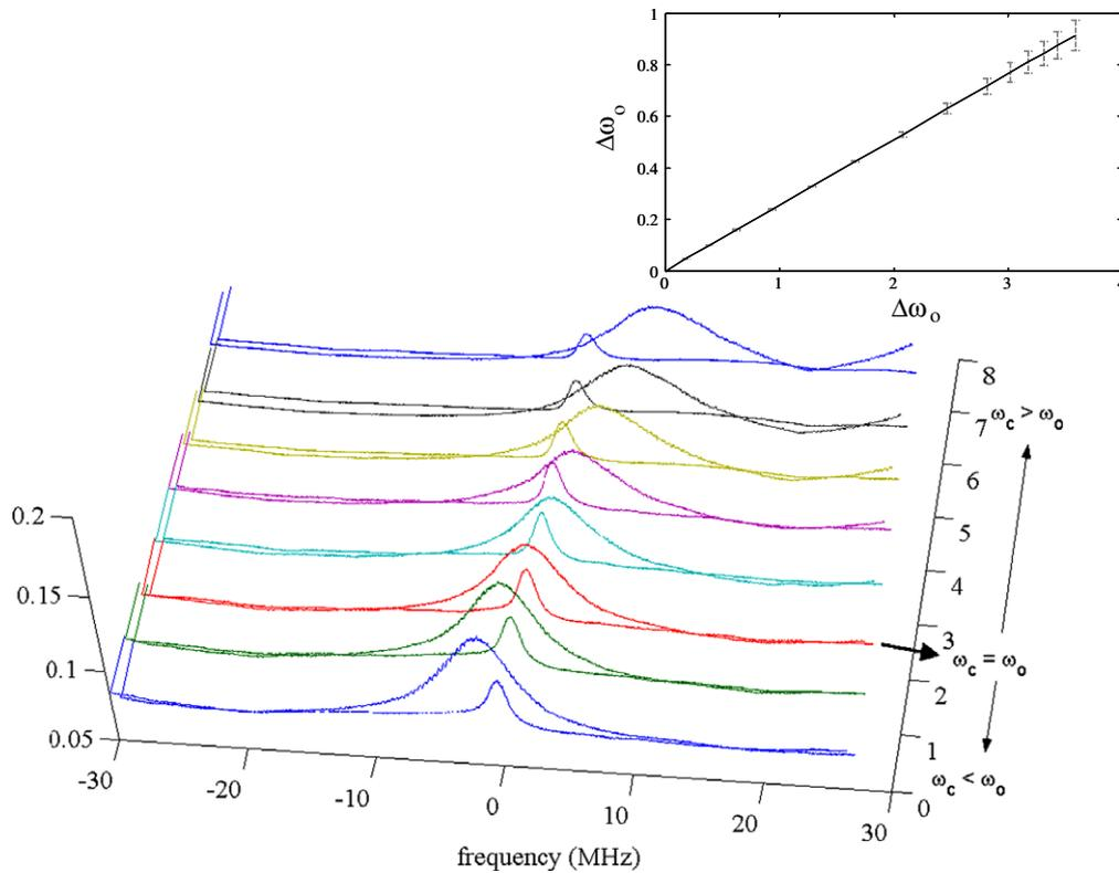
**Fig. 3.** Cavity resonances with (narrow) and without (broad) the effect of the intra-cavity medium dispersion. The inset in the figure shows measured frequency shifts corresponding to the peaks of resonances, illustrating reduced sensitivity to length change. The straight line superimposed on the data represents the fit to Eq. (2).
