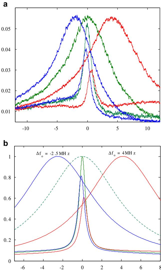
**Fig. 2.** (a) Experimental results showing linewidth narrowing and reduced shift in cavity resonance for  $\Delta f_0 = -2.5, 0$  and  $4$  MHz, respectively (b) theoretical model for cavity response (cavity linewidth =  $8$  MHz, EIT Linewidth =  $1$  MHz,  $L/\ell = 10$  and  $n_g \approx 50$ ). In the figures, the horizontal axis represents the frequency in MHz and the vertical axis represents the cavity transmission in arbitrary units.
