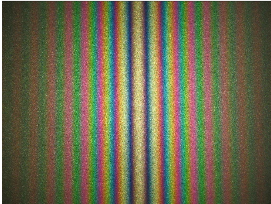
Fig. 1.1: Interference fringes resulting from white light propagating through a double slit. The m^{\text{th}} fringe for a particular wavelength \lambda is located at an angle \theta_m such that d\sin(\theta_m) = m\lambda , where d is the distance between slits.
